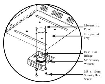
**Step 3.** Line up the mounting slots on the base box bridge with the mounting points on the equipment tray.
